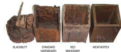
SAMPLES REMOVED FROM TERMITE TEST AFTER 2.5 YEARS EXPOSURE
